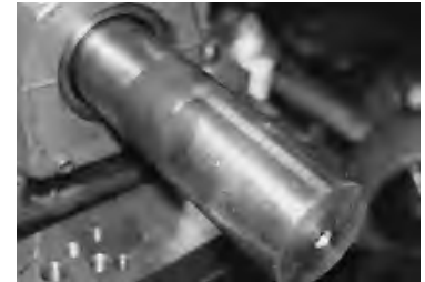
No fretting corrosion or shaft damage with Grip Tight Bearing Assembly.
